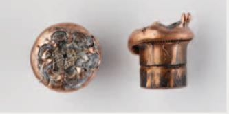
40 S&W FlexLock bullet fired through sheet metal (Glass and metal most difficult to penetrate deeply in target after passing through these two)
