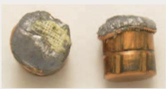
9mm FlexLock bullet fired through glass
