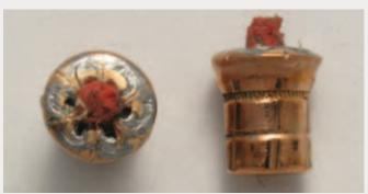
9mm FlexLock bullet fired through sheet metal
