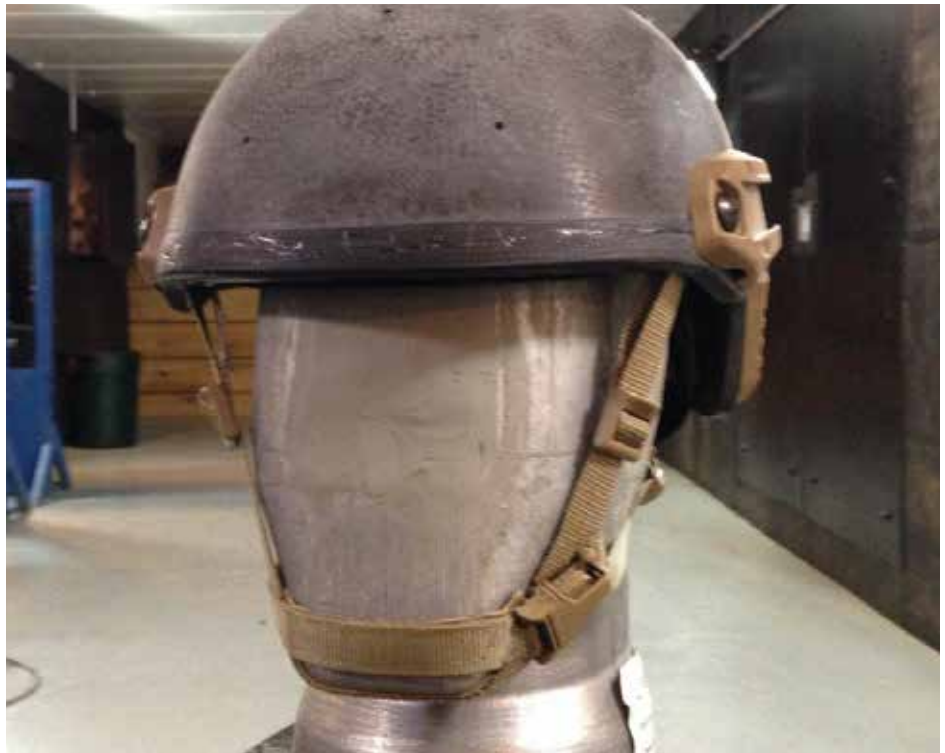
Helmet that has been prepared for ballistic penetration and backface deformation testing. (Photo courtesy of HP White Laboratory & Ops Core)
