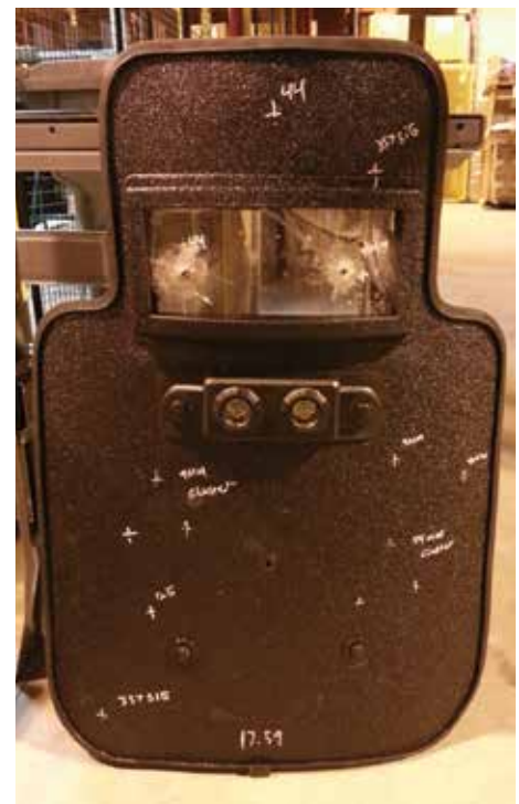
Ballistic shield after testing. (Photo courtesy of Ken Fuller, US Marshals)
